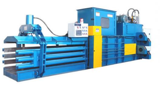
The recyclables are transferred into the baler's metallic hopper by means of a chain conveyor. Once the hopper is full of material, the baler's main piston runs forward and the material is entering the tunnel, thanks to the metallic plate's pressure. The working pressure has been pre-viously set at the desired value. Once the desired bale length is obtained, it is tied automatically with steel wire.
